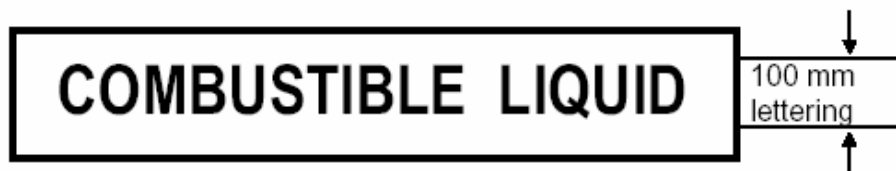
Figure 3 C1 combustible liquids placard
