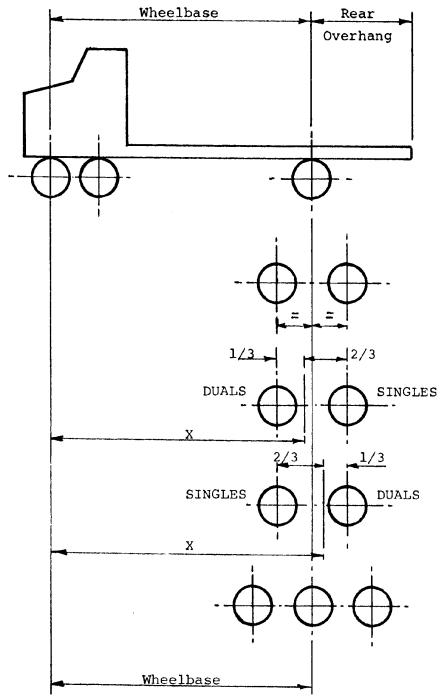
X = Distance from front'Axle' to the line from which the 'Rear Overhang' is measured.
