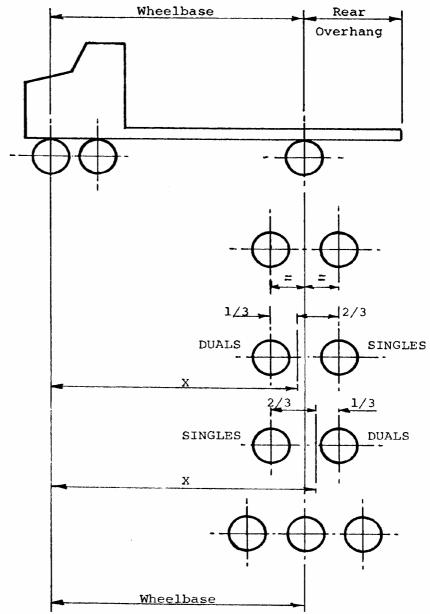
X = Distance from front'Axle' to the line from which the 'Rear Overhang' is measured.
