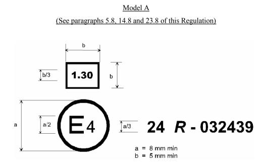
The above approval mark affixed to an engine/vehicle shows that, pursuant to Regulation No. 24, the engine/vehicle concerned has, with regard to the emission of visible pollutants by the engine, been approved in the Netherlands (E 4) under approval number 032439; the Regulation, at the time of approval, included already the 03 series of amendments. The corrected absorption coefficient is  $1.30 \text{ m}^{-1}$  (in the case of a vehicle approval).
