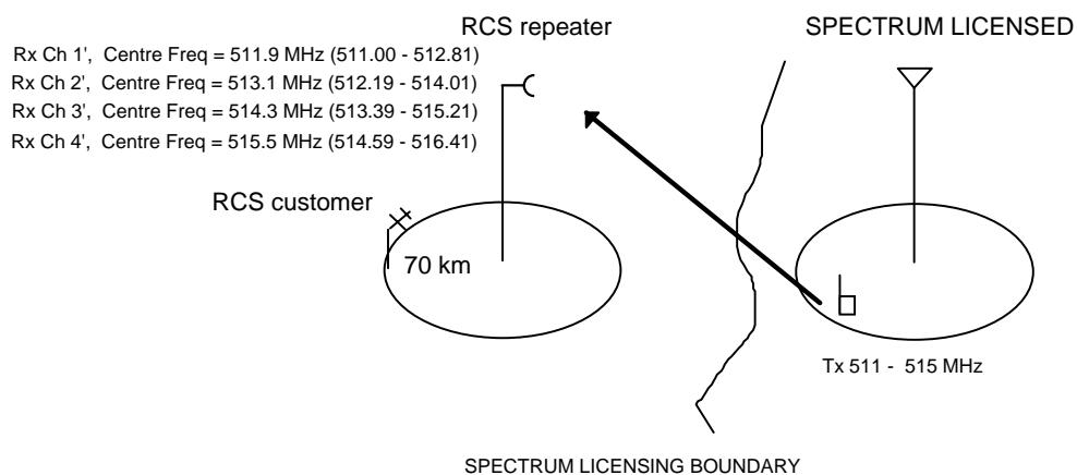
*RCS customer station receivers with centre frequencies 511.9 MHz (ch 1') and 514.3 MHz (ch 3')*
