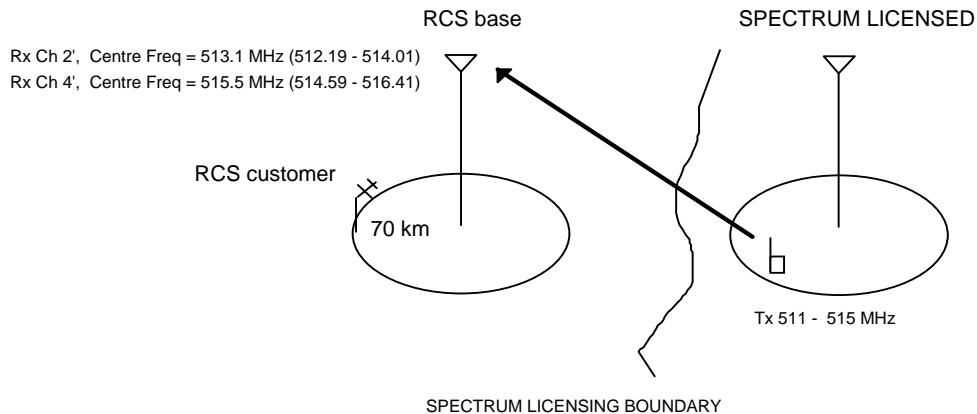
*RCS repeater station receivers with centre frequencies 511.9 MHz (ch 1'), 513.1 MHz (ch 2'), 514.3 MHz (ch 3') and 515.3 MHz (ch 4')*
