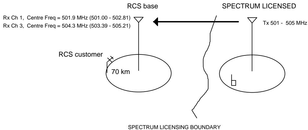
*RCS repeater station receivers with centre frequencies 501.9 MHz (ch 1), 503.1 MHz (ch 2), 504.3 MHz (ch 3) and 505.5 MHz (ch 4)*
