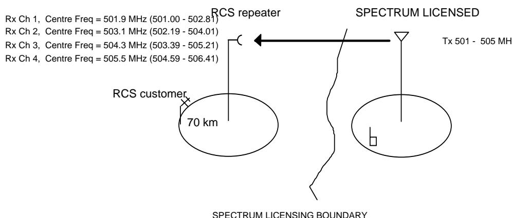
*RCS customer station receivers with centre frequencies 503.1 MHz (ch 2) and 505.5 MHz (ch 4)*
