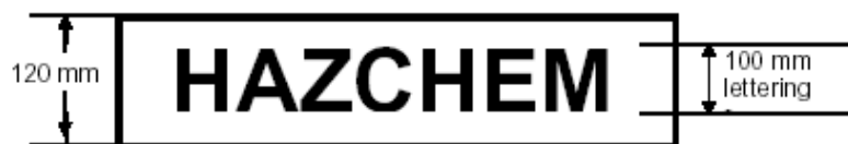
Figure 13.1 Form and dimensions of outer warning placard
