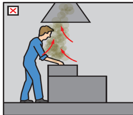
Diagram 5: Poor design carries through the breathing zone.
