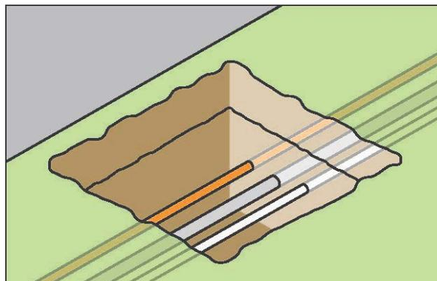
**Figure 1:** Underground essential services exposed by 'potholing'
