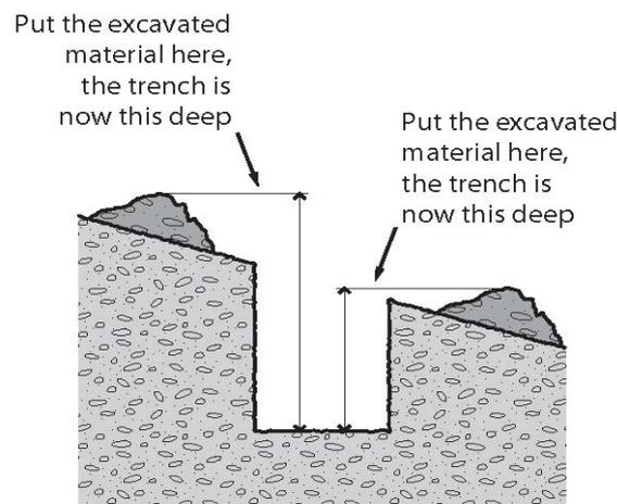
**Figure 3:** Excavated material impact on effective excavation depth
