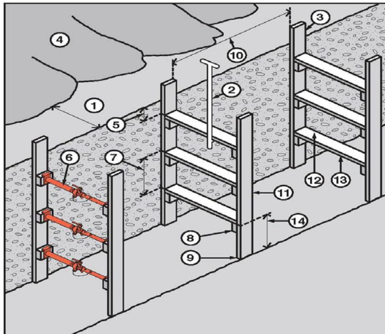
1. Spoil heap at least 600mm clear of excavation allows access along both sides of the trench top and prevents material from the heap rolling into the trench.
