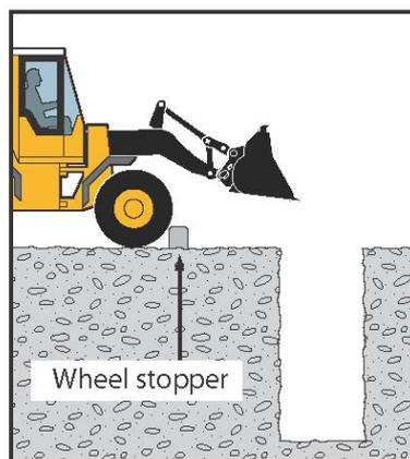
**Figure 5:** Preventing plant operation near excavations
