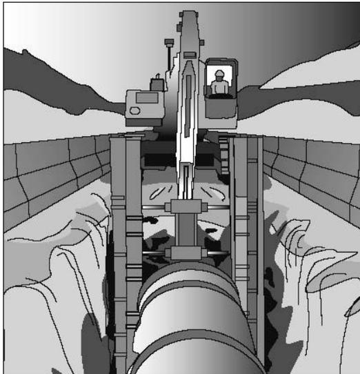
**Figure 6:** Extending trench shields above the excavation
