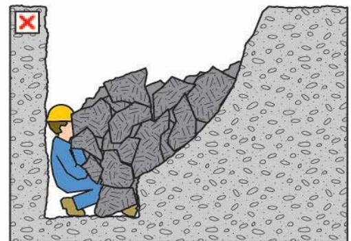
(d) Worker badly injured and probably smothered after being crushed against the opposite wall by the collapsing ground. The weight of a wedge of sand over a one metre length of trench two metres deep is about three tonnes
