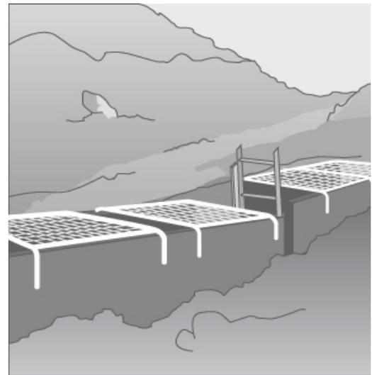
**Figure 7:** Steel mesh covers over trench shields
