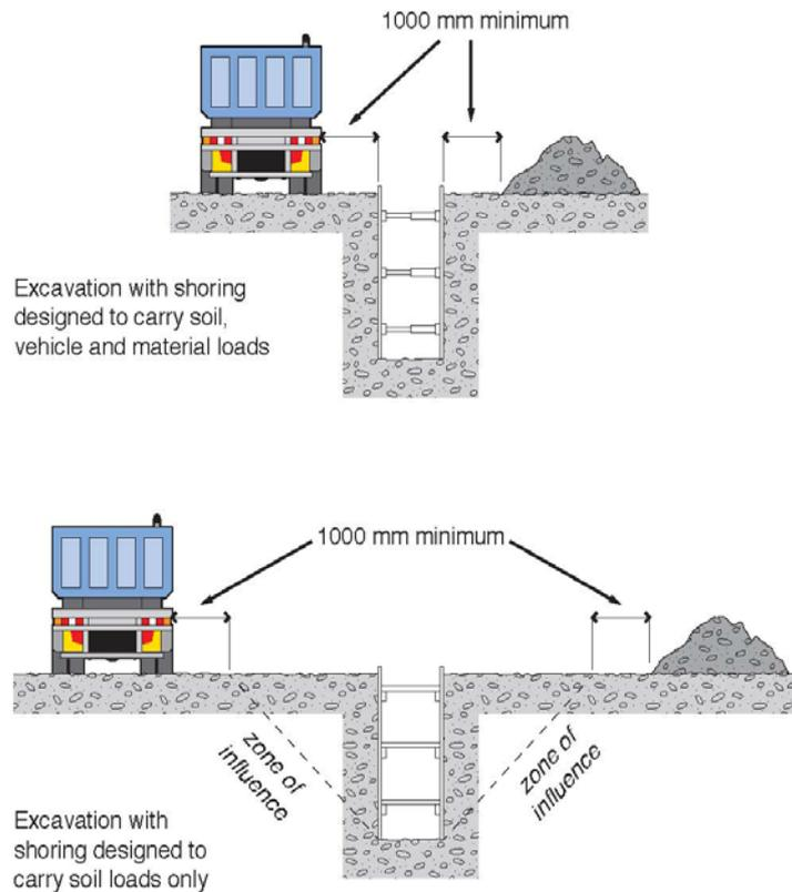
**Figure 2:** Excavated material and loads near excavations
