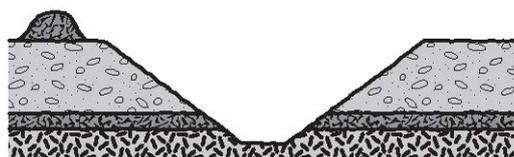
**Figure 10:** Battering
