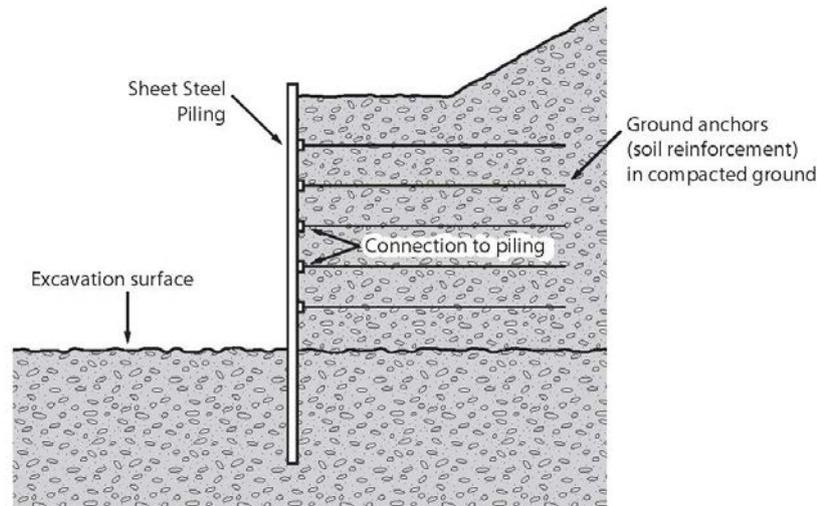
**Figure 18:** Ground anchors for supporting steel sheet piling
