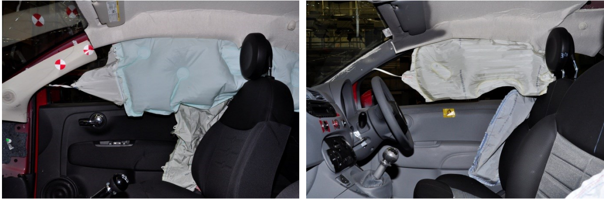
Figure 12 North American market vehicle (left) and Australian market vehicle (right) head curtain and thorax side airbags, post deployment (Model A)
