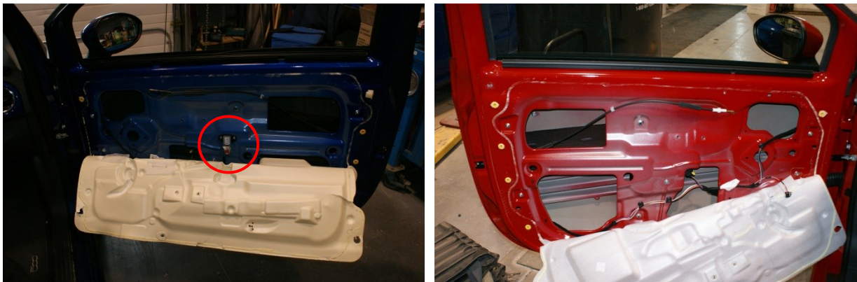
Figure 13 North American market vehicle (left) and Australian market vehicle (right) front-row door designs (note: pressure sensor (in red circle) fitted to the North American vehicle) (Model A)
