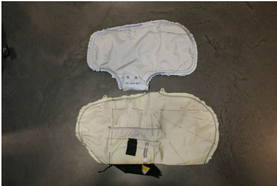
Figure 15 North American market vehicle (bottom) and Australian market vehicle (top) thorax side airbags (Model A)
