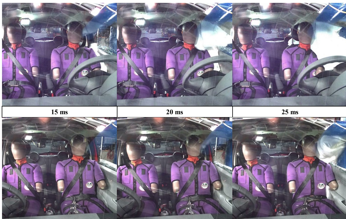
Figure 16 North American market vehicle (top row) and Australian market vehicle (bottom row) side airbag deployment, 15-25 milliseconds after first vehicle contact with the pole, during an oblique vehicle-to-pole side impact test (Model A)
