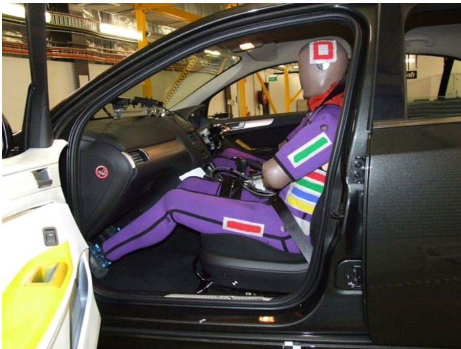
Figure 10 A WorldSID 50 th percentile adult male positioned in a large passenger car
