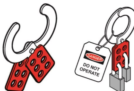
Figure 3 Example of tag and lockout with the padlocks of two workers.
