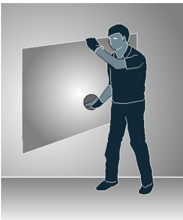
Figure 26 Use handling grip devices adapted to the particular object to be carried
