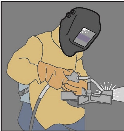
Figure 3 Welder wearing welding helmet, dry leather welding gloves and leather apron
