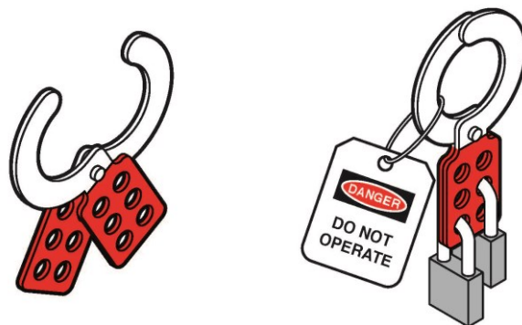
Figure 9 Example of lock-out with a tag and the padlocks of two workers
