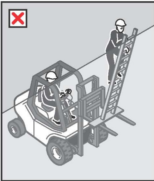
Figure 14: Unacceptable practice with ladder on forklift.
