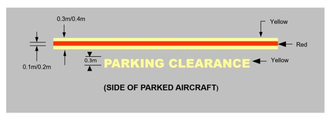
Figure 8.50 (5) Parking clearance line (shows matters)
