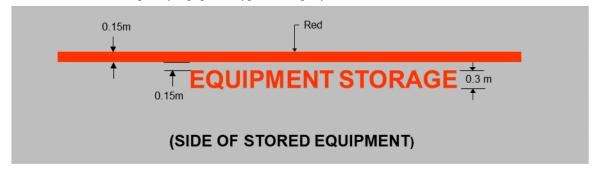
Figure 8.53 (4) Equipment storage and apron road marking (illustrates matters)
