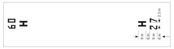
Figure 8.116 (2) Helicopter FATO designation marking and heliport identification marking for a runway type FATO (shows matters)
