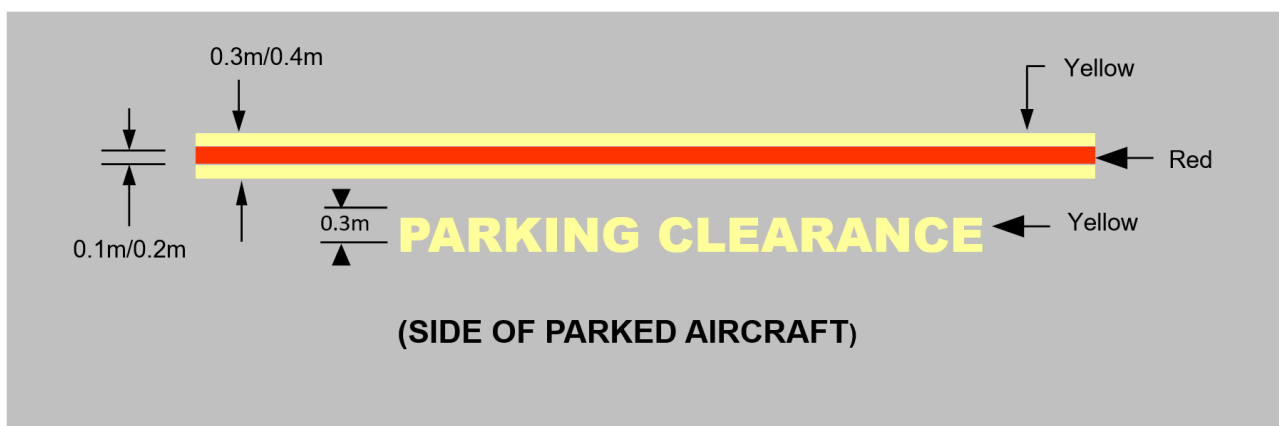
Figure 8.50 (5) Parking clearance line (shows matters)
