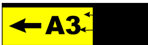
Figure 8.98 (2) Runway exit sign (illustrates matters)
