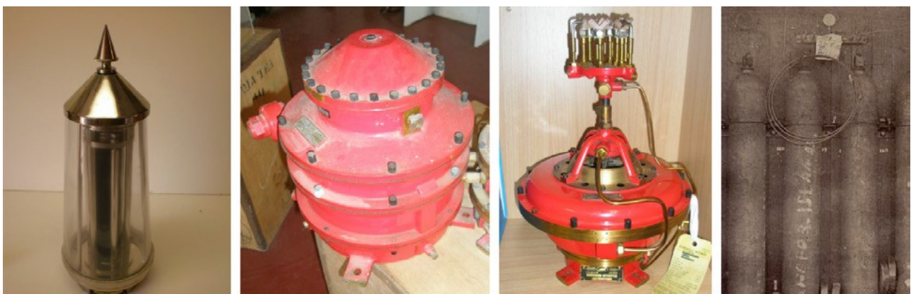
Figure 13. Dalén's system – sunvalve, mixer, flasher and cylinder
