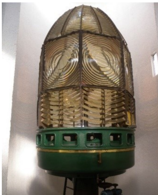
Figure 12. Dioptric lens on display at Narooma
