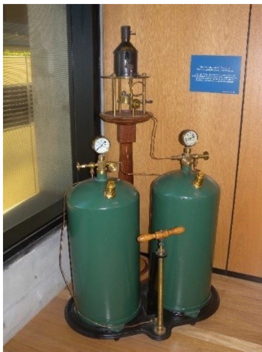
Figure 11. Incandescent oil vapour lamp by Chance Brothers
