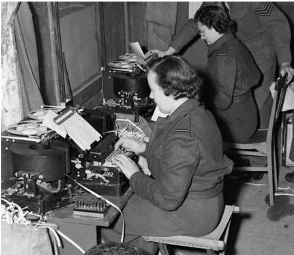
Figure 39 Typex cypher machines of the type housed in the Dugout, operated by the Women's Auxiliary Air Force (UK)
