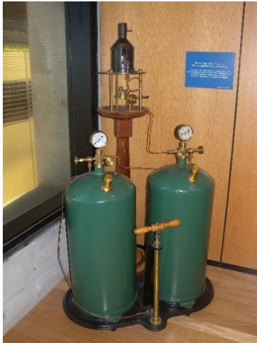
Figure 8. Incandescent oil vapour lamp by Chance Brothers (Source: AMSA)
