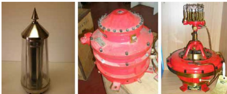
Figure 10. Dalén's system – sunvalve, mixer, flasher (Source: AMSA)
