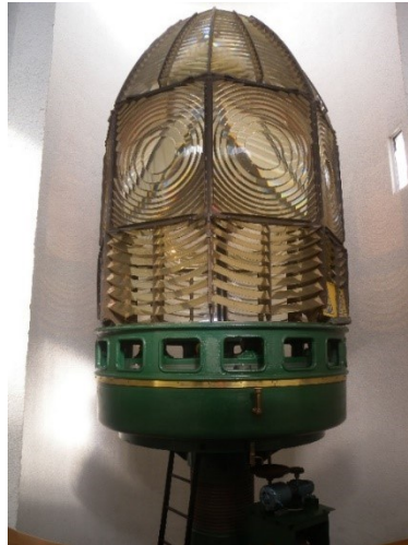
Figure 9. Dioptric lens on display at Narooma (Source: AMSA)
