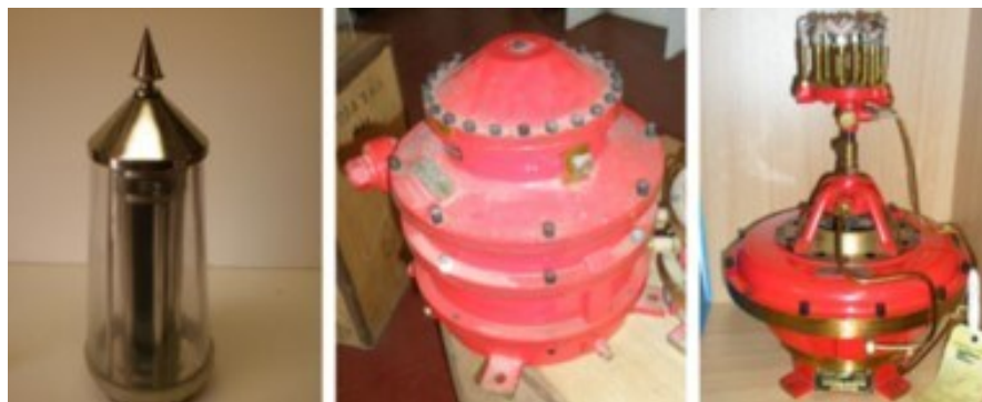
Figure 12. Dalén's system - sunvalve, mixer, flasher and cylinder (Source: AMSA)
