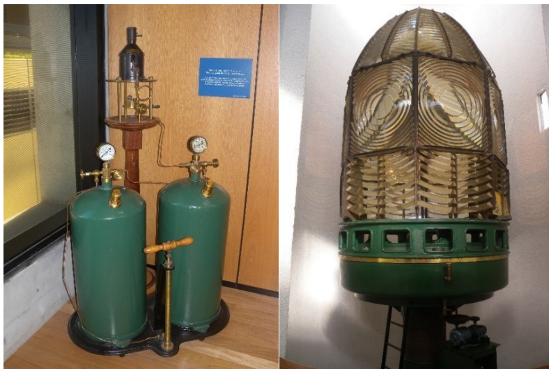
Figure 10. Incandescent oil vapour lamp by Chance Brothers (Source: AMSA)
