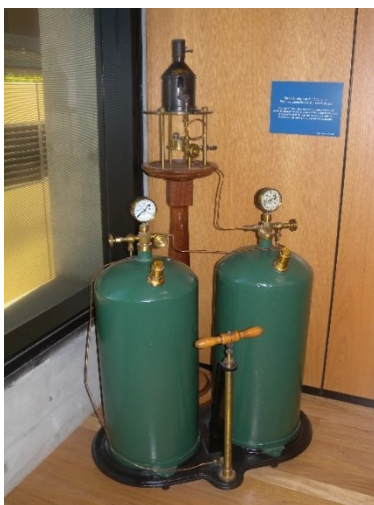
Figure 9. Incandescent oil vapour lamp by Chance Brothers (Source: AMSA)
