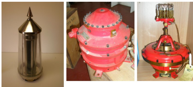
Figure 11. Dalén's system – sun valve, mixer and flasher (Source: AMSA)
