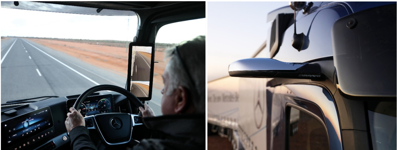
Figure 1: An internal monitor (left) and external camera (right) of a camera-monitor system for indirect vision (source: supplied by Daimler Truck and Bus Australia Pacific)
