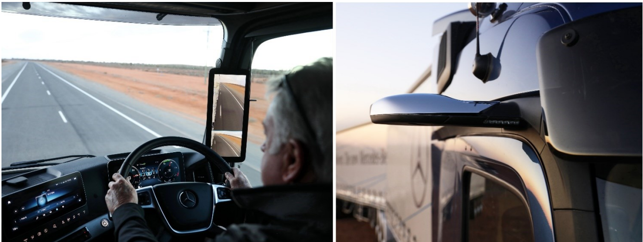
Figure 1: An internal monitor (left) and external camera (right) of a camera-monitor system for indirect vision (source: supplied by Daimler Truck and Bus Australia Pacific)
