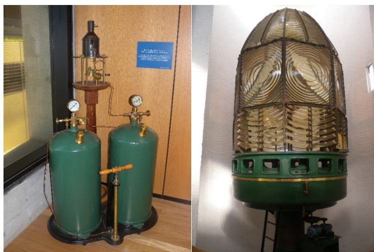
Figure 9. Incandescent oil vapour lamp by Chance Brothers (Source: AMSA)
