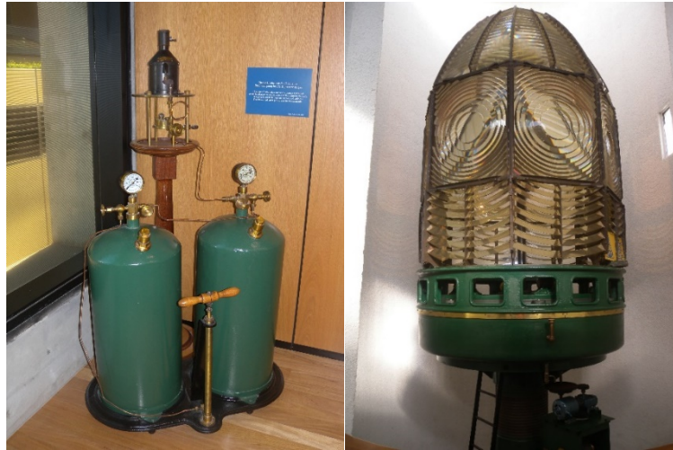
Figure 8. Incandescent oil vapour lamp by Chance Brothers (Source: AMSA)
